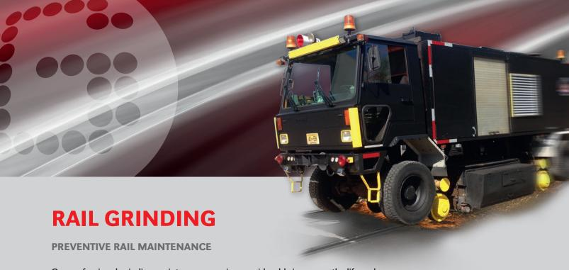
Our professional grinding maintenance service considerably increases the life cycle of rails as well as lowers noise emissions from train operations. We machine rails and switches efficiently and precisely using modern road-rail vehicles.
