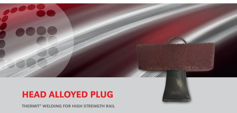
The pouring system distributes micro-alloys in the head of the rail supplied by a patented plug. It greatly improves the hardness and subsequent wear resistance of the weld on the running surface while keeping the base ductile. It can be used on AREMA High Strength rail steels, compatible with a range of common rail profiles and with any 1" Orgo-Thermit kit you currently have in stock. The achievable hardness range in the rail head is 370 BH  $\pm$ 0.
