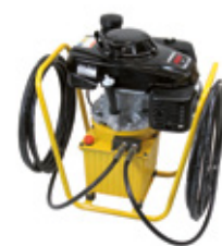
Hydraulic pump driven by 4-stroke engine type Honda
