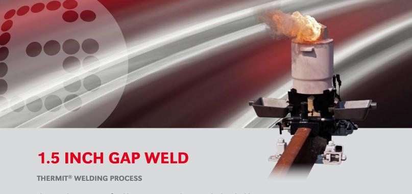
The 1.5 inch gap THERMIT® welding process is used as a standard method for joining of steel rails for specifically heavy haul applications in some countries. The increased gap width from a 1 inch gap width allows for a reduced solidification rate for additional time for reaction gases and impurities to escape from the weld mass.
